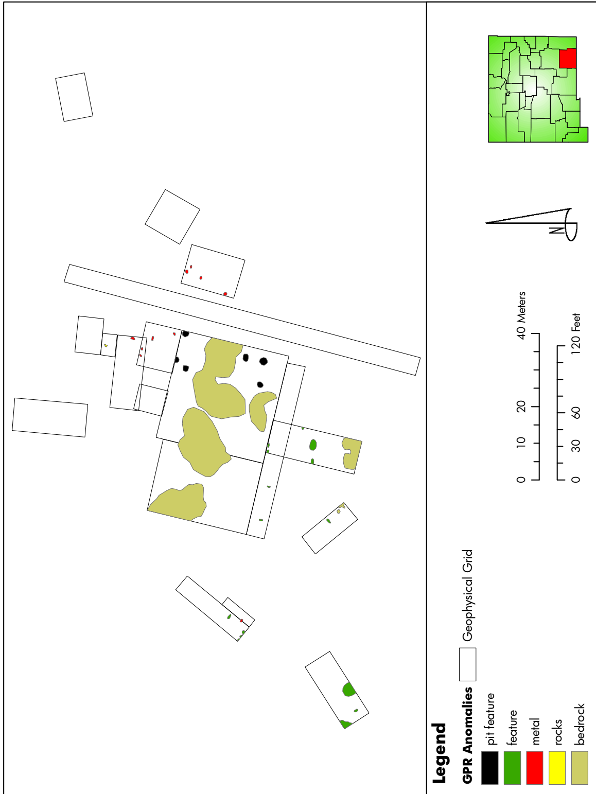
Figure 6. Map Showing GPR Anomalies in the Survey Grids
