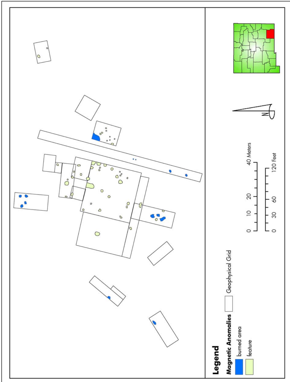
Figure 6.3 Composite map showing magnetic anomalies in the survey grid
