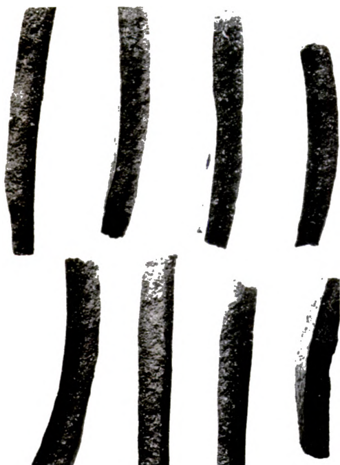
FIGURE 28a Cross sections of culinary vessel walls. The clay is heavily carbonaceous. Repeated use over cooking fires has burned out carbonaceous material, leaving a darker band on the interior.
